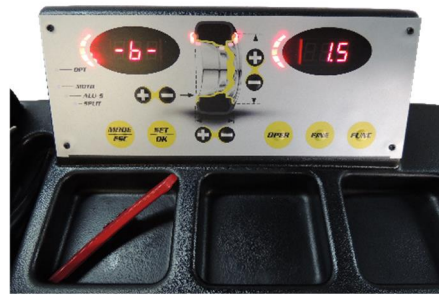
Balancer LED Digital Display & Storage Tray
