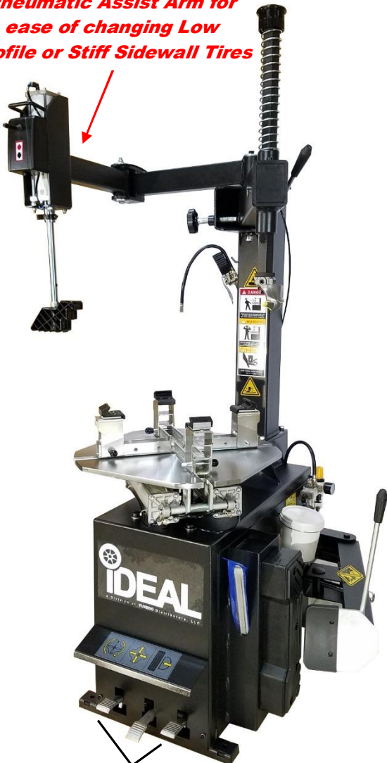
Simple Foot Pedal Operation for Table Rotation, Clamping & Bead Breaking
