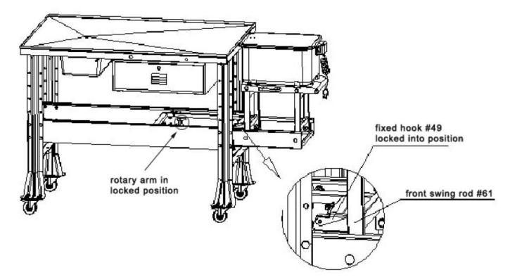
5. To store Parts Washer when not in use, release the Fixed Hook (49), then raise the Rotary Arm Lever to the vertical position to unlock and then lower the Parts Washer to the rack and slide it under the tabletop. Once the Parts Washer is stored below the tabletop, lower the Rotary Arm Lever to the horizontal position to lock the Parts Washer in place.
