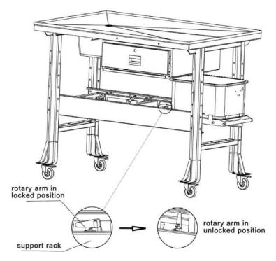
2. Once the Parts Washer has been released from the locked position, slide it out from under the tabletop. Do this by pulling the Handle on the front of the Parts Washer Tray. Once the Parts Washer is fully extended, then lower the Rotary Arm Tab into the rear locking hole on the support rack, so that its locked in the extended position.
