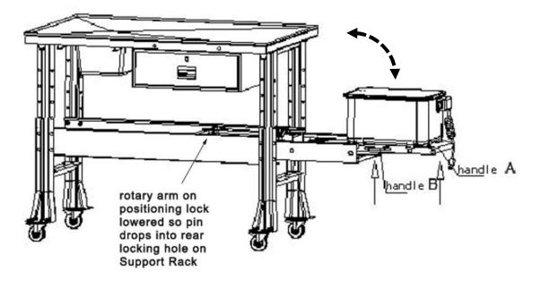
Flip the Fixed Hook (49) down and place the head of the Hook Insert into the hole of Front Swing Rod (61) to assure stability and to lock the Parts Washer into the operating position.
