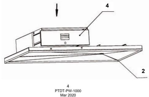
4. Assemble the Drawer (4) with the Fixed Mounts to Tabletop.
