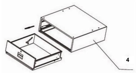
3. Attach the Fixed Mounts (A & B) to the Drawer Shell (4) with Bolts, and then carefully insert Drawer into the Shell.
