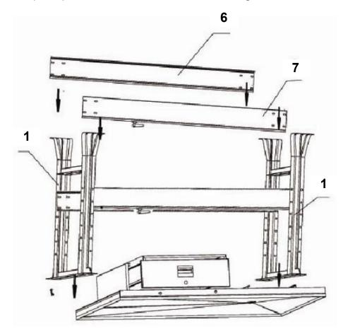
6. Carefully rotate the assembled Table with Leg Assemblies (1) and Support Rails (6 & 7) in the upright position.
