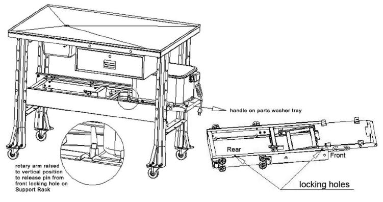
3. Next, raise the Parts Washer using **Handles (A & B)** until the swing rods supporting the Parts Washer are in the vertical position and Parts Washer is positioned against tabletop.
