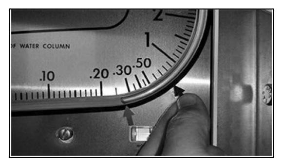
At this point, your manometer is set up and ready to use. You should never need to move the arrows once they are placed. Always check the manometer before turning the fan on to ensure the red fluid is sitting on the 0 mark. If the fluid is not on 0, turn "Zero Set" knob to adjust fluid to zero before starting fan.
