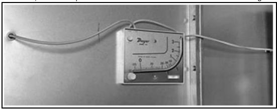
1. Drill a hole in booth wall just large enough for the plastic hose barb to fit through (approx. 13/32). Install washer and nut on back side. Do not over tighten.
