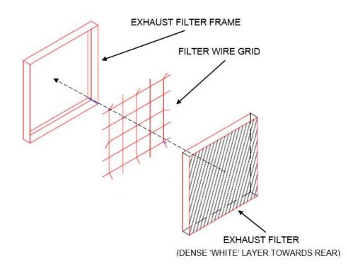
(NOTE: Install Exhaust Filters with the green shaded color towards inside of Booth)
